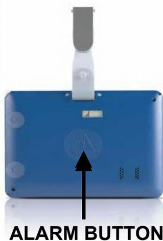
On the back of the card is a button that can be pressed if the holder feels at risk. When pressed the alarm automatically opens a phone line to a control room. The control room immediately listens to what is going on, and if they feel it is necessary then they will call the police. They have a direct line to the police which is quicker than going via 999. The ID card then vibrates like a mobile phone regularly so that the user knows that the police are on their way.
